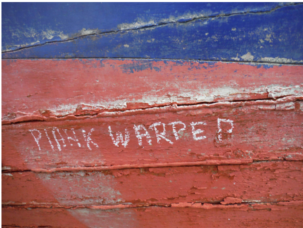
WARPPED PLANK STARBOARD SIDE 6 NOTE CONDITION OF SEAMS
