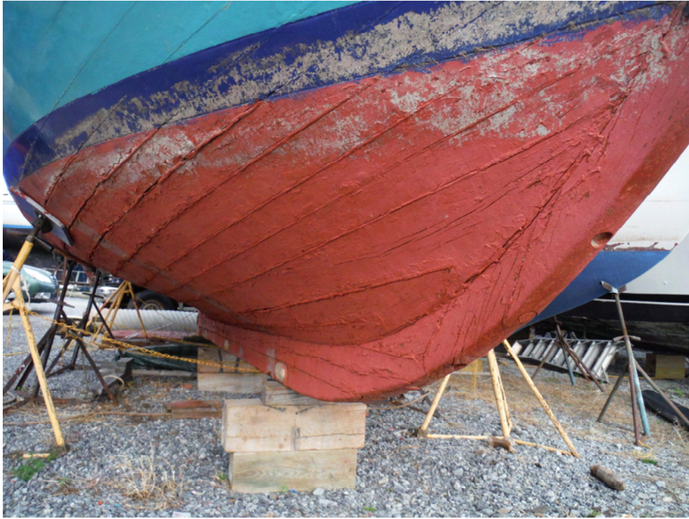
FORWARD VIEW OF BOTTOM 6 NOTE SEAMS
