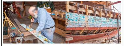
The Woody has been stabilized with the installation of new shear clamps, bilge stringers, and the new king plank as the professional shipwrights are shifting their attention to the Clearwater.
